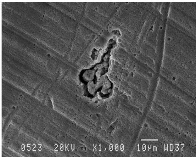
Fig. 11 Surface appearance for sample (S5) after 600 s exposure to 10% aqueous solution of \text{HNO}_3 + \text{Fe}_2(\text{SO}_4)_3 concentrate at room temperature. Note typical pit structure with jagged edges and particle remnants within the pit (1000 \times )
